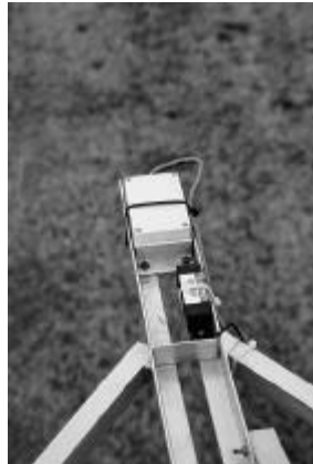
Figure 1. The Watson FGM-301 three-axis fluxgate magnetometer was installed on an aluminum frame mounted above and behind the tractor cab.
