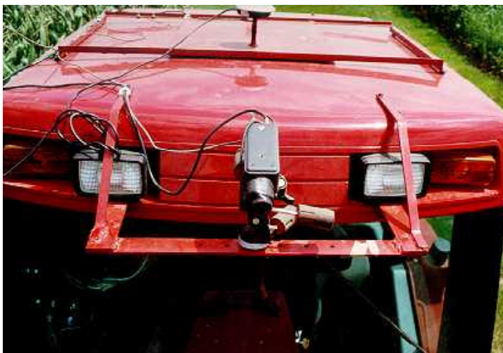
Figure 8. Mounting of the Elmo vision sensor
