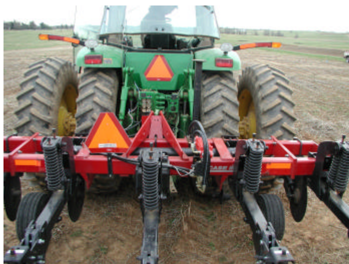
Figure 1. Design team modifications to the subsoiler enables prescriptive, site-specific tillage depths.
