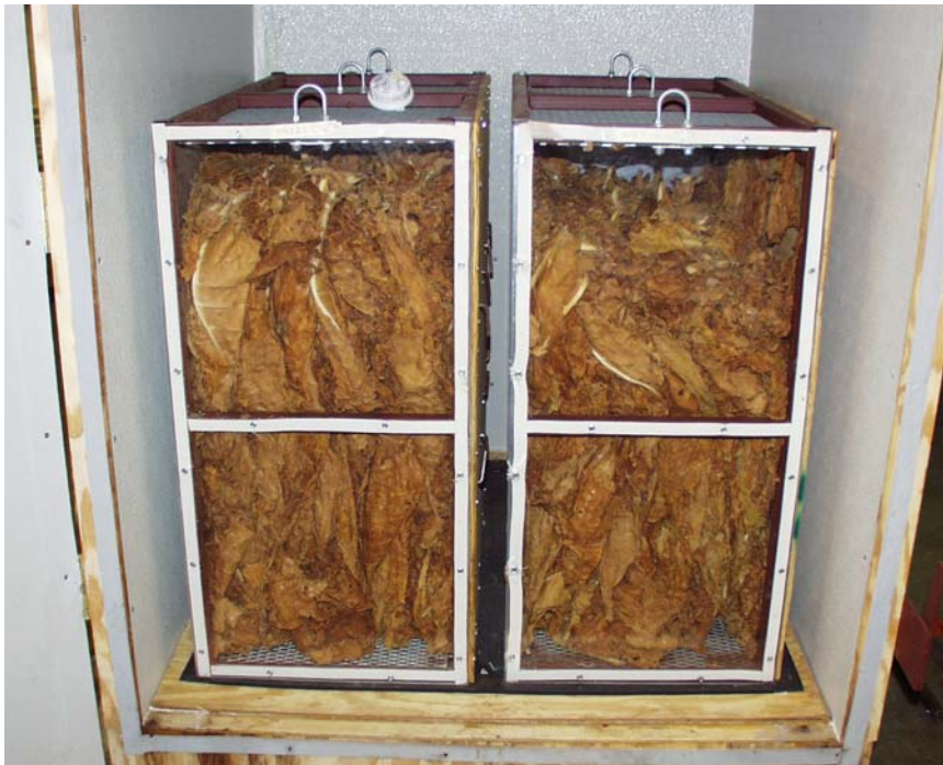
Fig. 6. View of metal boxes with plexiglass front in laboratory environmental chamber used for leaf curing trials.
